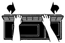
8. Slide the top of the vent cover into place. Push the bottom until it snaps into place. Replace the mounting screws. Turn the power back on at the main power supply.
