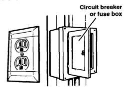
If your electrical power line or outlet voltage is less than 110 volts, cooking times may be longer. Have a qualified electrician check your electrical system.
