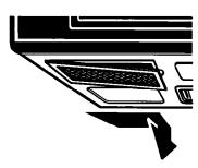
To remove grease filters, slide each filter to the side. Pull filters downward and push to the other side. The filter will drop out.
