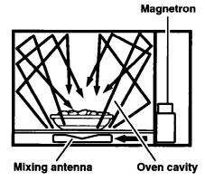
A magnetron in the microwave oven produces microwaves. The microwaves move into the area under the oven floor. There they bounce off the mixing antenna into the oven where they contact the food.
