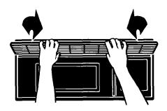
Slide the bottom of the vent cover into place. Push the top until it snaps into place. Replace the mounting screws.
