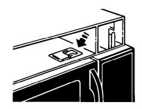
4. Remove bulb holder mounting screw.
